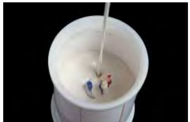
Pour the investment material slowly. Avoid the formation of air bubbles.
