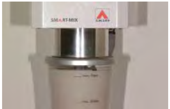
Mix IPS Empress Esthetic Speed Investment material under vacuum. Check the vacuum.
