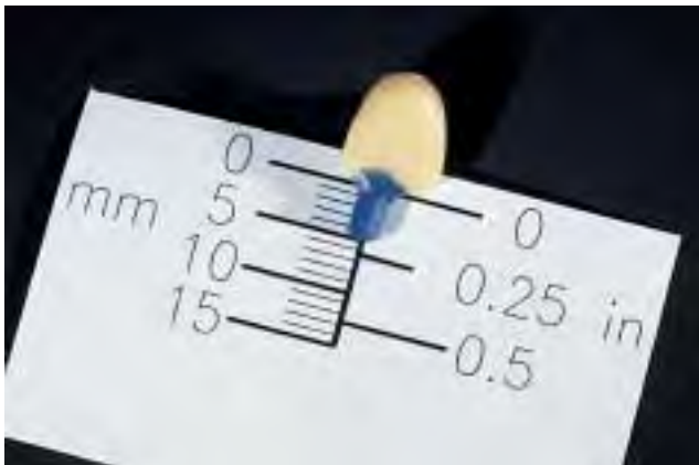
Length of the sprues: 3 mm to max. 8 mm
