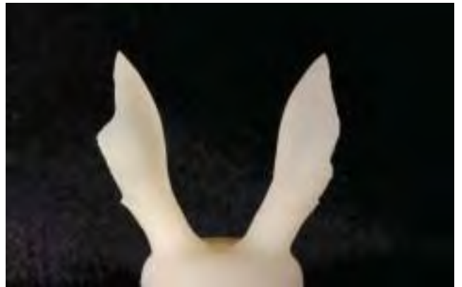
Veneers after pressing in the EP500/EP600/EP600 Combi according to the IPS Empress Esthetic press parameters.
