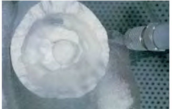
Rough divestment is carried out with Ivoclar Vivadent Polishing Jet Medium at 4 bar (60 psi) pressure.
